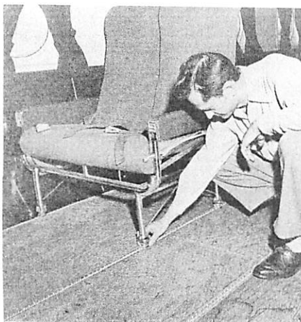
All Series G Track Fittings can be operated easily with one hand and locked into the track.
